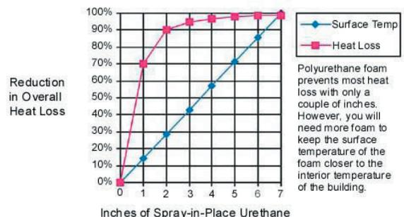
The graph shows that 70% of heat loss from conductance is stopped by a one inch thickness of spray-in-place urethane foam. Remember we are going to stop nearly 100% of the heat loss from
